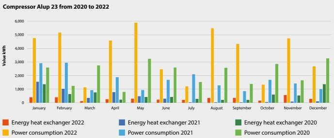
Unfortunately, it was detected only during the evaluation that the heat exchanger had recovered significantly less process waste heat in percentage terms than in previous years. The analysis in the technical department revealed that only one of the two pumps was working. This deficiency has now been remedied.
