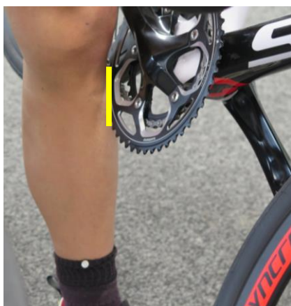
Pict. 11: Contact with the front gear rim of a racing bike tilted to the left
