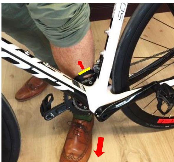
Pict. 12: My reconstruction attempt with the (chainless) large front gear rim which is located at the right side of the bicycle. Red arrows: if the leg is moving to the front an upwardly directed injury occurs.
