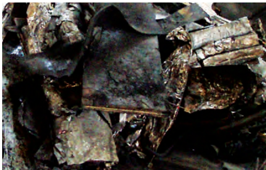
This is what happens when pedelec batteries go bad, which is why retailers need to know how to properly store and charge them.
