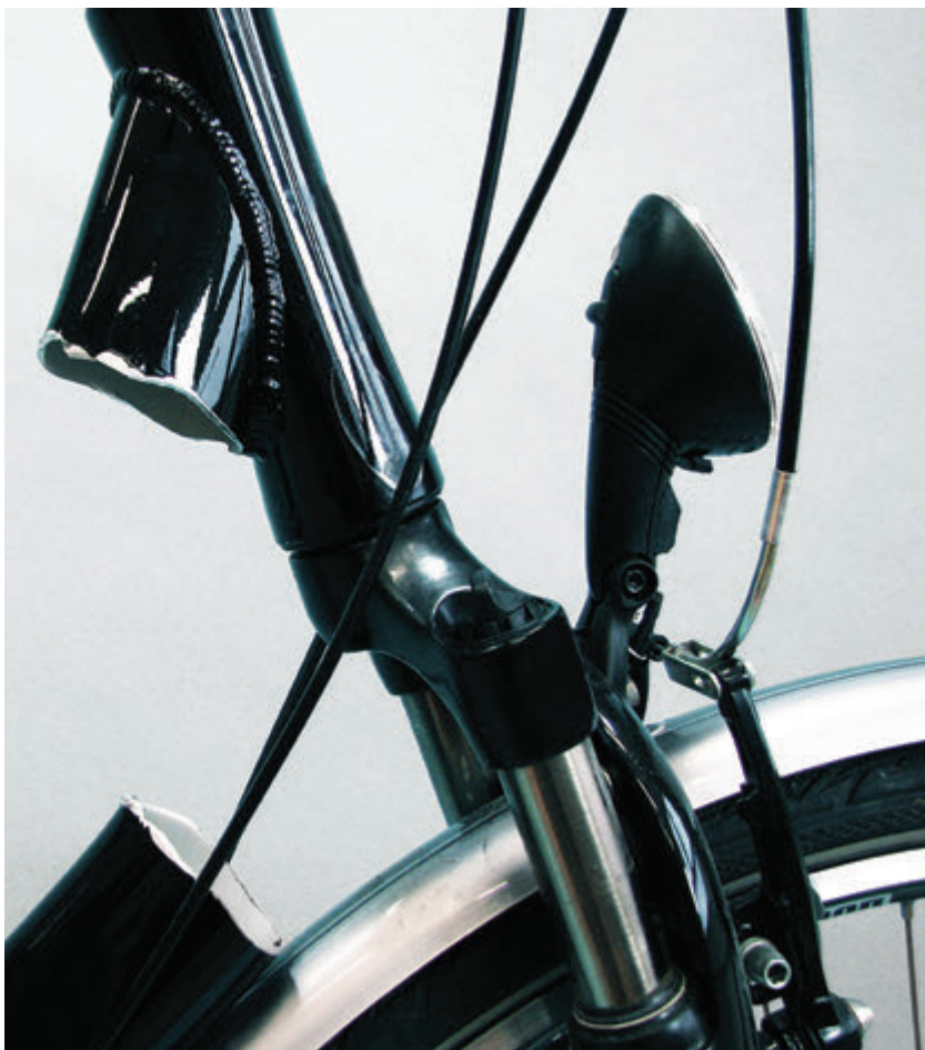
A broken frame on a step-through pedelec
